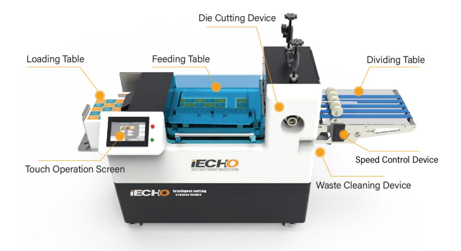
The equipment has the functions of uninterrupted automatic feeding, automatic paper feeding, automatic deviation correction, double-sheet detection, marking and alignment die-cutting, and automatic waste discharge.
